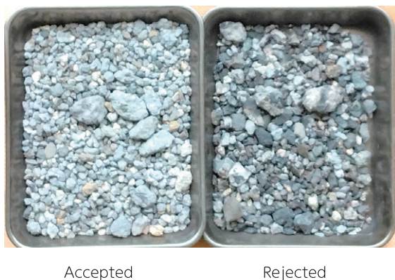
Fig. 10 Appearance of color-sorted raw material for green refractory products.
